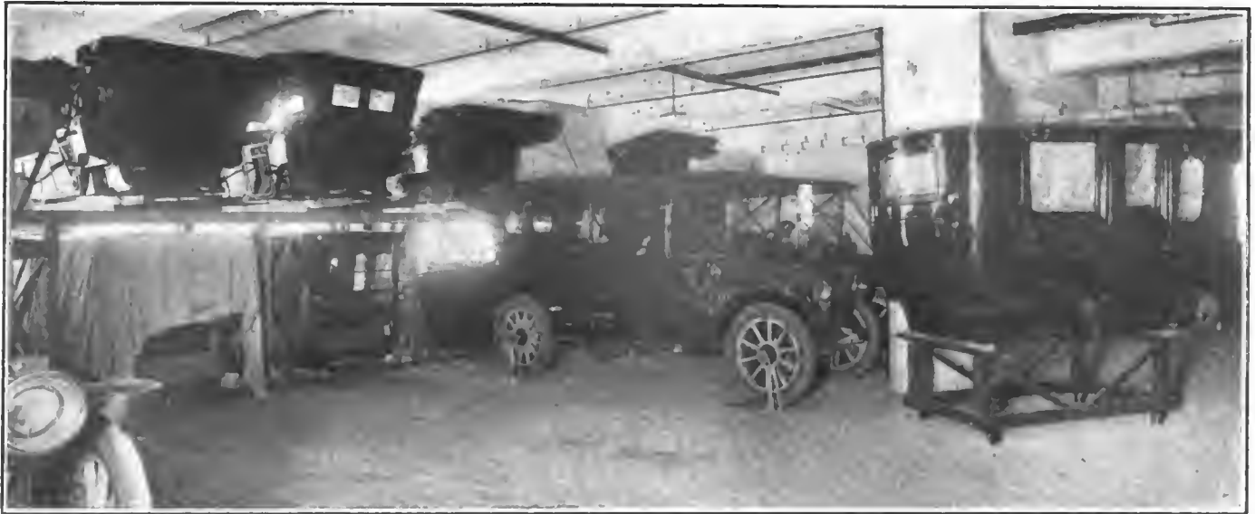
Fig. 8—View in the dead storage department. Racks are provided for the storage of two tiers of bodies, as shown
